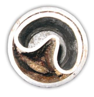
Cut steel pipe showing PTFE lined collapse through blocked vent holes
