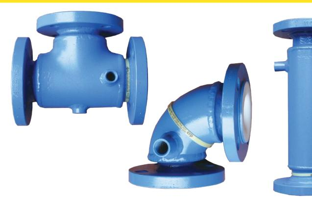
It is possible to provide a source of heating or cooling to a lined piping system by using jackets around the equipment. Here the core pipe is completely surrounded by a jacket pipe. The process material travels through the lined pipe as normal, whilst the heating or cooling medium travels through the outer jacket.
